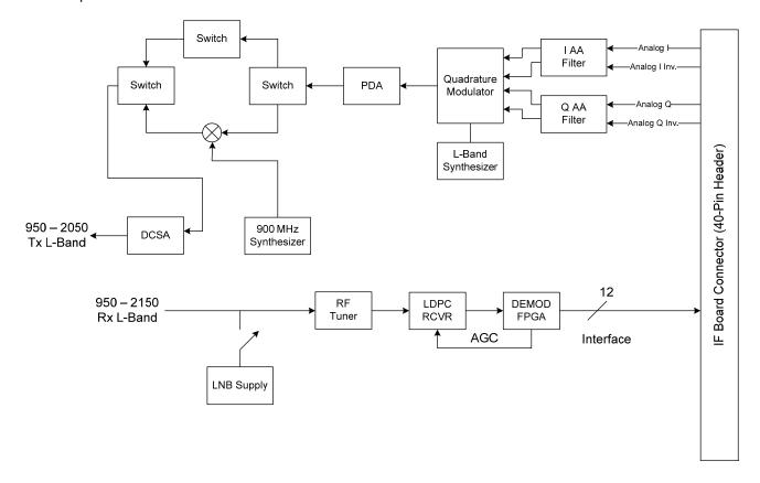
Figure 3-2. IF Card Block Diagram
