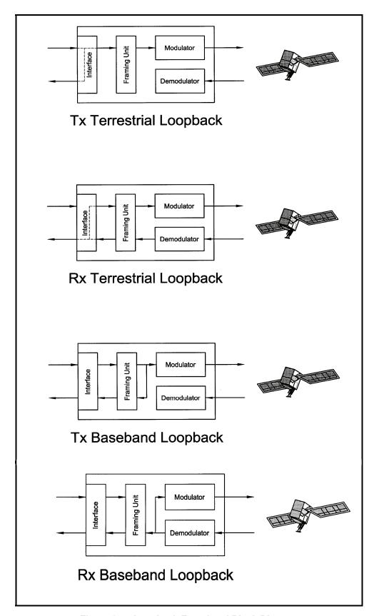
Figure 3-5. Loopback Functional Block Diagram
