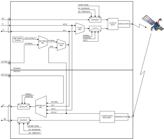
Figure 3-6. Clocking and Polarity Diagram
