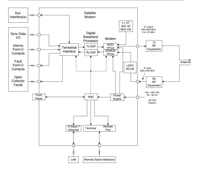
Figure 3-3. Satellite Modem Functional Block Diagram
